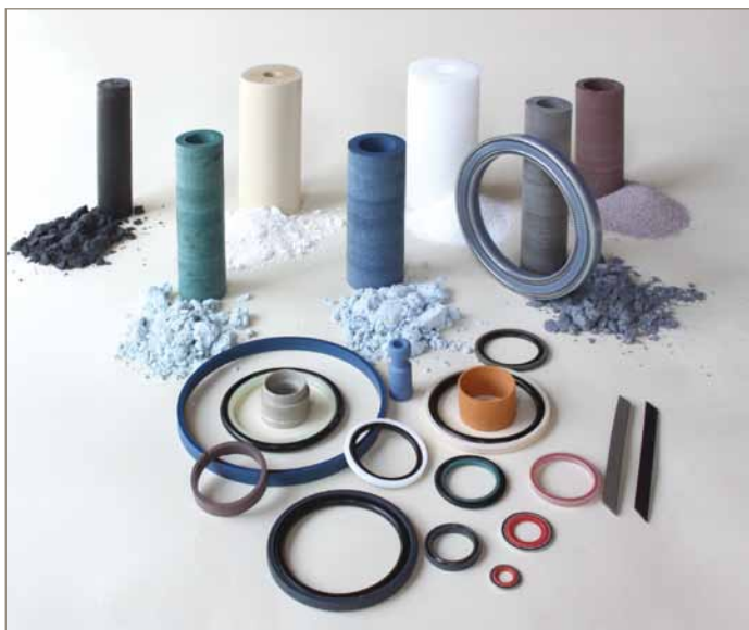
Fig. 2.3 – PTFE powder, semi-finished shape and final machined product.
